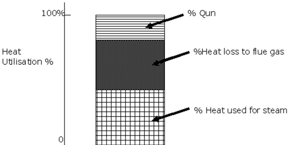
RESULT: Hence A test is conducted on the boiler and the equivalent evaporation capacity and its thermal efficiency are determined. Also a heat balance sheet is drawn.
